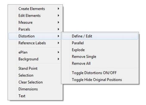
GeoCivil contains a data structure which enables elements to have multiple locations; a true position and a distorted position. This is particularly useful in creating "surveyor's fieldnotes" for lodgement at the Land Titles Office, etc. In situations where a plan drawn to scale is crowded, elements can be moved to provide more "white space". GeoCivil will draw the elements in their distorted positions but adopt the dimension of the true positions.
