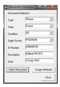
Note that to check that a feature has been correctly attributed hover the cross hair over the feature so that a temporary popup appears showing the features attributes. The right arrow key on the keyboard can be used to scroll through other features in the vicinity of the curser.
