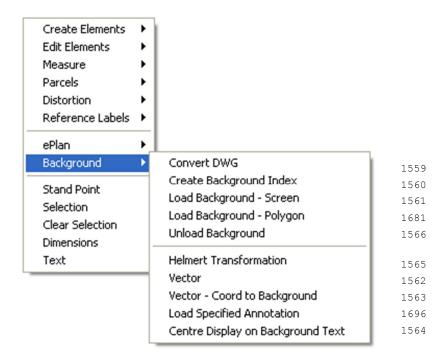
Note: The **Background** functionality is setup to display the Victorian cadastre as background to your project data. It converts the DWG format tiles to a GeoCivil format and displays the relevant tiles. This can be readily modified to accommodate any form of background graphics.
