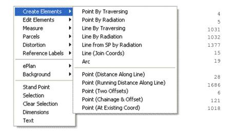
Point By Traversing - creates a Point element of the current feature by bearing and distance from the current Standpoint. The new Coord becomes the Standpoint.
