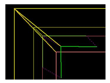
The above screen grab shows the distorted NW corner achieved by first "exploding" the related Coords by a factor of 5 then individually dragging some Coords. The dashed lines show the individual distortions; the thicker lines being the distorted positions. The display of distortions is controlled from the **Configure Display** tool.
